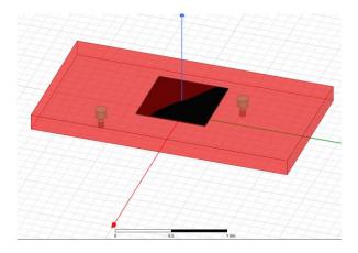
The absorber type is ECCOSORB MCS. There are two effects of absorber in the cavity. The first is that the presence of any material in the cavity will lower the cavity resonance frequencies. Absorber in general has high permittivity ( $\epsilon$ ) and high permeability ( $\mu$ ). From inspection of the cavity resonance equation shown previously, permittivity or permeability greater than 1 will lower the resonant frequencies.
