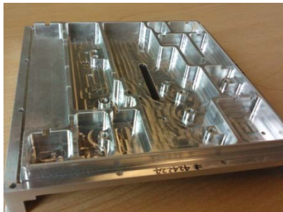
Figure 1: A typical machined aluminum chassis prior to FIP dispense
