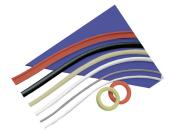
Conductive elastomers are ideal for automotive applications requiring both environmental sealing and EMI shielding. Compounds can be supplied in molded or extruded shapes, sheet stock, and custom extruded or die-cut shapes to meet a wide variety of applications. Conductive elastomers provide shielding effectiveness up to 120dB at 10GHz. Conductive extrusions offer a wide choice of profiles to fit a large range of applications.
