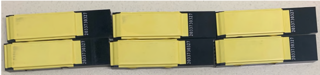
6 heat sink samples, DX4, DX5, DX6, DX10, DX11, DX12 with adhesive lot #18115
