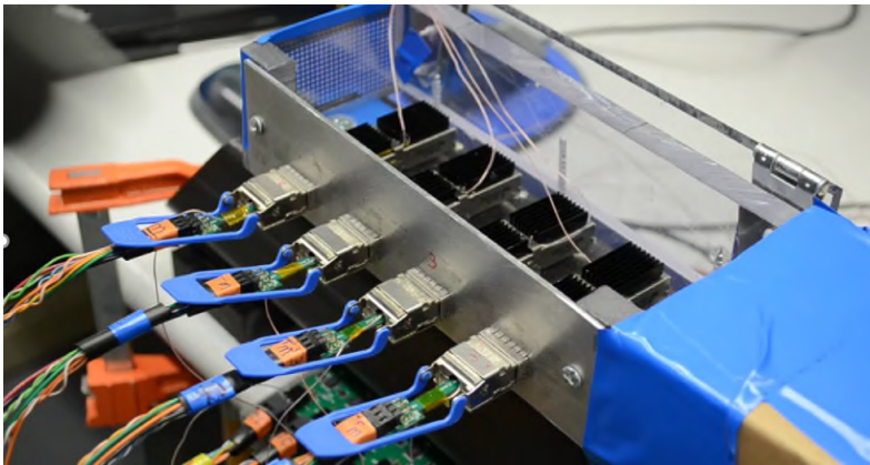
QSFP-DD, 4 position test setup using Molex cage and heatsinks.
