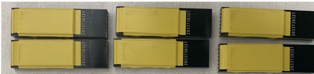
6 heat sink samples, DX16, DX17, DX18, DX22, DX23, DX24 with adhesive lot #19124
