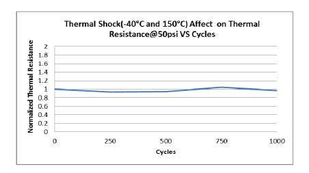
Graph5&6 indicate that Tgard500 maintains its thermal, and dielectric qualities after exposure to 1000 thermal shock cycles between -40  $^{\circ}$ C and + 150  $^{\circ}$ C.
