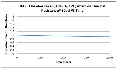
Graph1, 2 show the results of HAST chamber aging effect, the dielectric properties of Tgard500 were not obviously affected by the exposure to 85 % relative humidity and 85  $^{\circ}$ C after 1000 hours, and the thermal resistance at 50psi was stable with time increase, and it was slightly reduced within 10% range at 50 psi and then eventually stabilizes as time of exposure increases.
