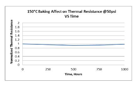
Graph3&4 showed that dielectric properties and thermal resistance at 50psi were stable during the 150 °C baking testing and maintained its thermal, and dielectric qualities.
