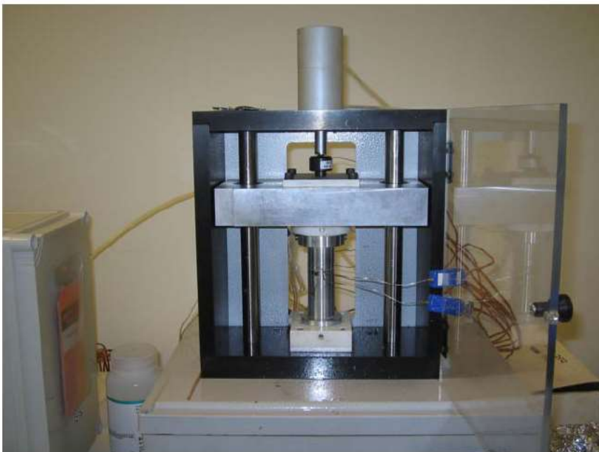
Figure 11: ASTM D5470 Thermal Resistance Tester
