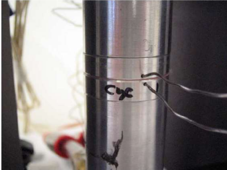
Figure 11: ASTM D5470 Thermal Resistance Tester
